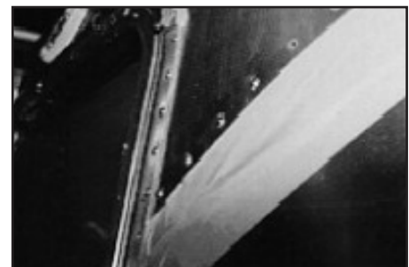
3. SHAVED BULB-TITE RIVETS MATCH SOLID RIVETS PERFECTLY!
