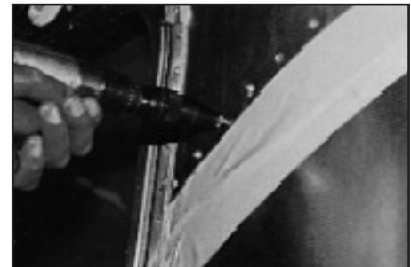
2. PROPER SIZED SHAVER TOOL, INSTALLED IN A STANDARD 1/4" DRILL, SHAVES RIVET HEAD.
